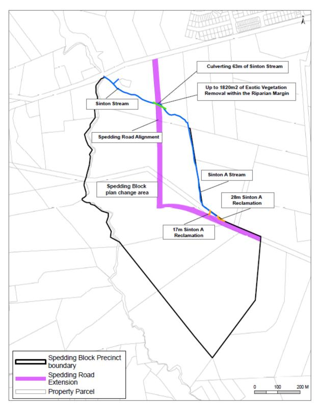
I616.9.2 Name: Precinct plan 2 - Stream and vegetation enhancements required for reclamation, drainage and vegetation clearance to enable the construction of Spedding Road (mitigation)
